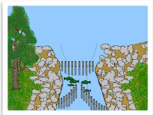
A fish weir is a fish trap, a stacked stone wall which is built across the riverbed in a large V-shape, to cleverly funnel and trap large numbers of fish in a small, walled area so that they can be easily netted or speared.
